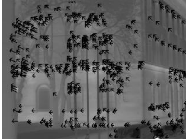
Fig. 1. IR image with selected SIFT features, that have correspondences in the following image. Arrows show the moving direction of the points
