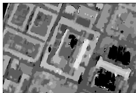
Figure 2. Digital surface model calculated for a section of 600 m \times 400 m from the Munich scene using the “dynamic line warping” approach
