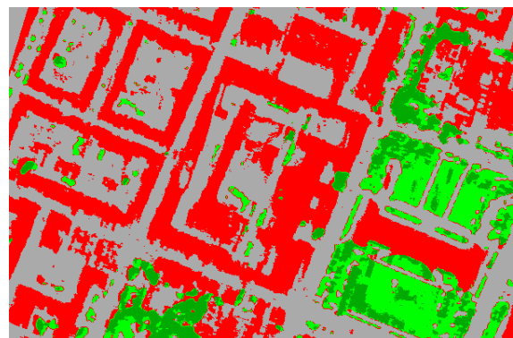
Figure 6. Classification of the Munich scene using a height mask derived from DSM and DTM and a vegetation mask based on the NDVI from the pan-sharpened orthophotos
