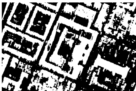
Figure 4. High objects mask calculated from the DSM and the derived DTM applying a height threshold of 4 m (section 600 m x 400 m)
