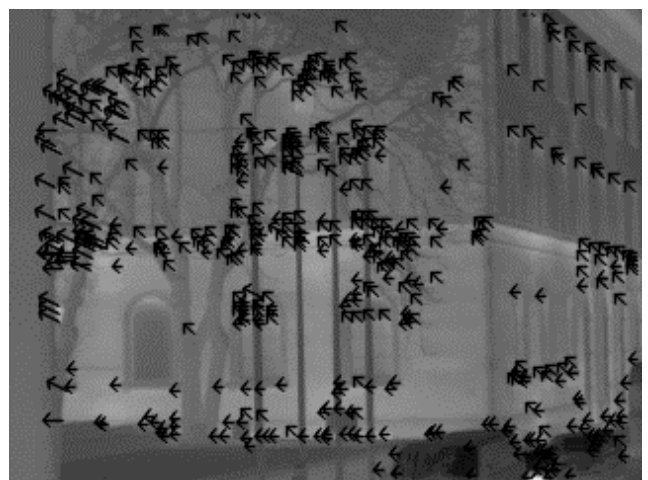
Figure 3. IR image with selected points of interest, that have correspondences in the following image. Arrows show the moving direction of the points.
