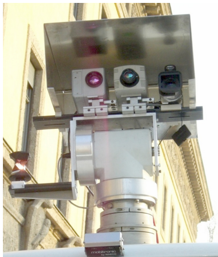
Figure 1: Used camera system: midwave (3-5 \mu\text{m} ) and the longwave (8-12 \mu\text{m} ) infrared camera (see the left and middle camera) and video camera right
