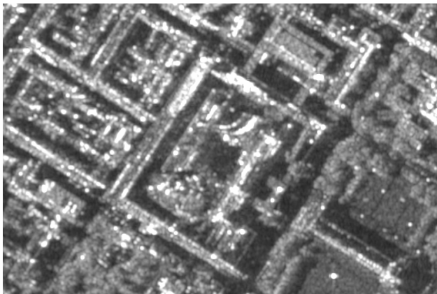
Figure 2. SAR image of the urban area in Fig. 1. The radar flight trajectory is aligned with the bottom side of the image. The image was taken with the E-SAR System (DLR-HR).
