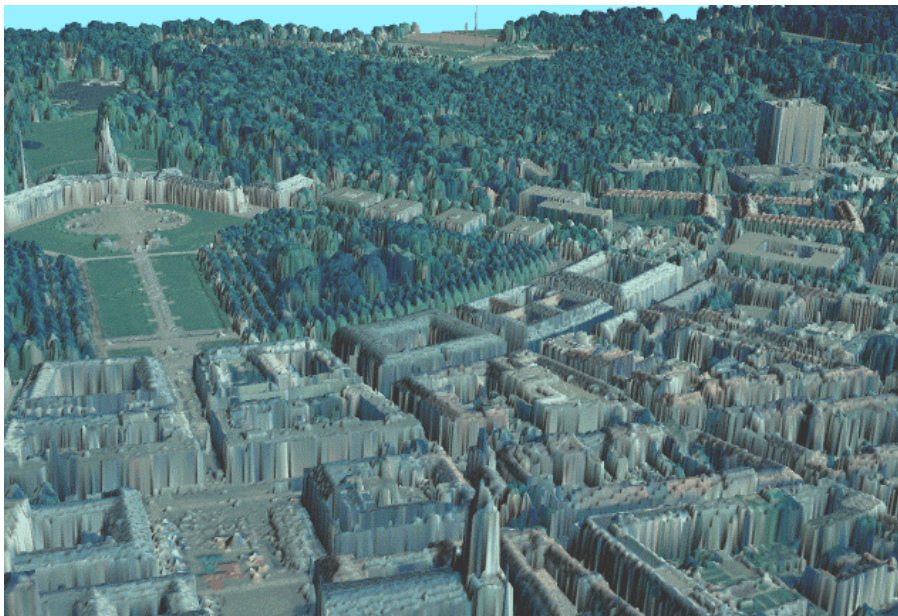
Fig. 3. 3D view of laser altimeter data textured by an aerial image.
