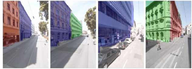
Figure 1: Four examples of automatically segmented street side images into individual building facades. Use is being made of overlapping street-side images. In this example, the camera is pointed forward (from Recky M. et al., 2011).
