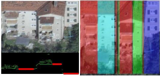
Figure 7: Plane detection for a complex facade; (a) key-view of a facade and projection in xy-plane (red lines are strongly weighted (>66% of points lie in this plane)); (b) determined major facade planes (segmented areas with balconies are marked in red)
