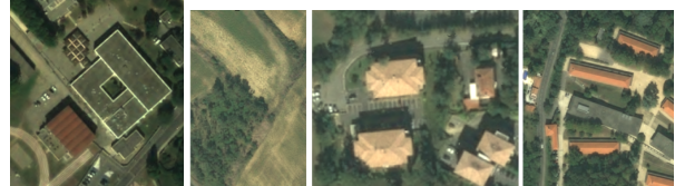
Figure 1: Radiometric information is not sufficient to distinguish classes with similar radiometry, such as grey roofed buildings from roads, or red tiles from bare soil.
