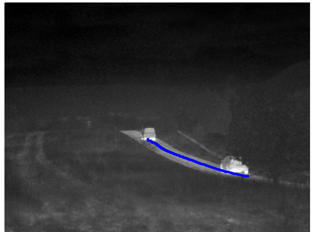
Figure 4: Same image as in figure 1. Here a two-dimensional track, as it resulted from the application of the IRST-algorithm to the whole image-sequence of camera C_V , is overlaid. The track belongs to the 'object' that had been marked with a blue rectangle in the center of figure 1.
