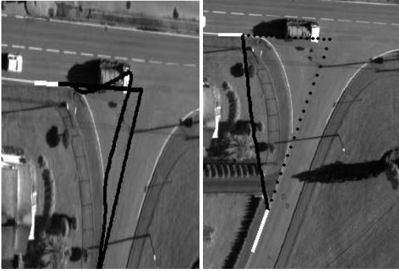
Figure 10. In (a), snake spacing is 2 pixels, which signifies dense vertices, and the accuracy of convergence is 1/10 pixel. Active contours are caught in the shadow cast by the truck. In (b), snake spacing is 12 pixels and the accuracy of convergence is 1/200 pixel. The optimized active contour (black line) cannot delineate the junction border.
