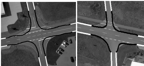
Figure 8: Ziplock snake optimization using tradition force field as an external force. Black curves are the result of snake optimization. White lines are the extracted road arms. Since the capture range of the external force field is small, the iterations are stopped near the initial positions.
