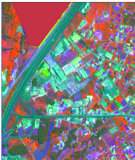
Figure 4: RGB-421 colour composite derived by decorrelation stretching of the IKONOS image bands.
