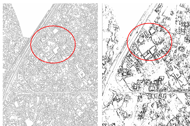
Figure 5: Left: The EDISON output edge map. Indicatively, an area with buildings is delineated with a red ellipse. Right: The Bezdek output edge map. The same area as in the left image is delineated with a red ellipse on the right image.
