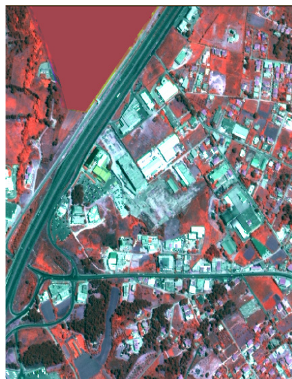
Figure 1: Pseudocolor composite RGB-421 of the IKONOS VHR image with spatial resolution of 1m-resampled and size 934x1070 pixels.
