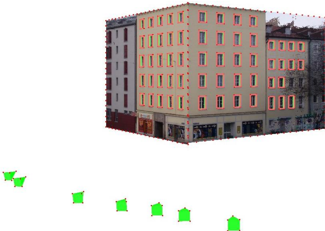
Figure 10: Result for sequence Ostbahnhof-1 (images cf. Figure 9) – Window outlines for three facades with rows of windows as red rectangles, 3D window positions as green rectangles, camera positions as green pyramids
