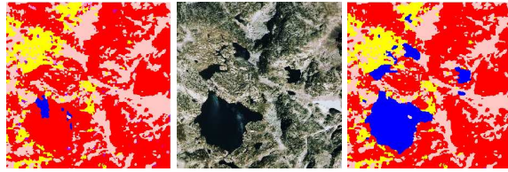
Figure 8: Results without (on the left) and with (on the right) prior information about shadows (rocks in red, screes in pink, pasture in yellow, water in blue)
