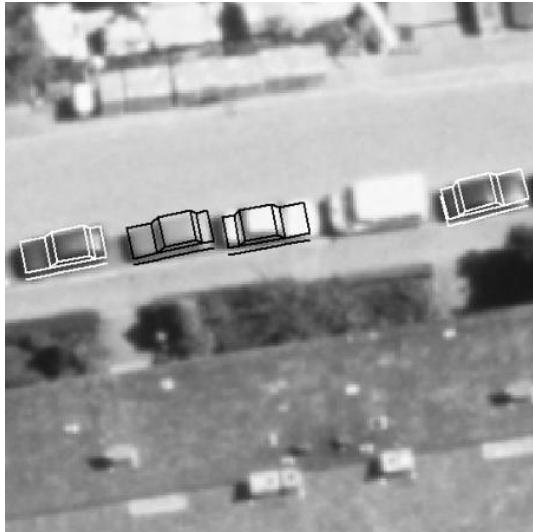
Figure 5: Detected vehicles: White wire-frame = Vehicles declared as dark during matching and vice-versa.
