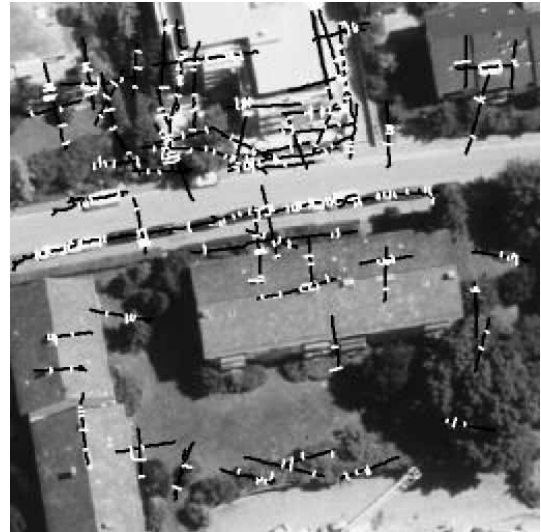
(a) Symmetry lines (SL, black) and intersecting edges (IE, white)
