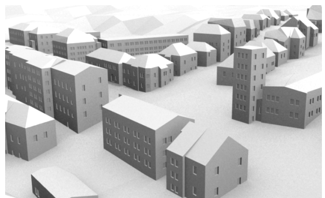
Figure 10. Facade geometry synthesized from grammar library
