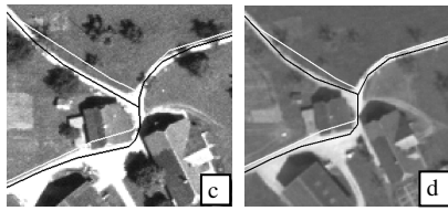
Figure 3. Examples of road extraction and junction generation in scenes with small settlements.
