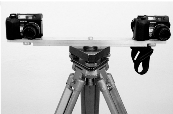
Figure 2. The photogrammetric base equipped with a pair of the Olympus C-4040 cameras placed on a tripod
